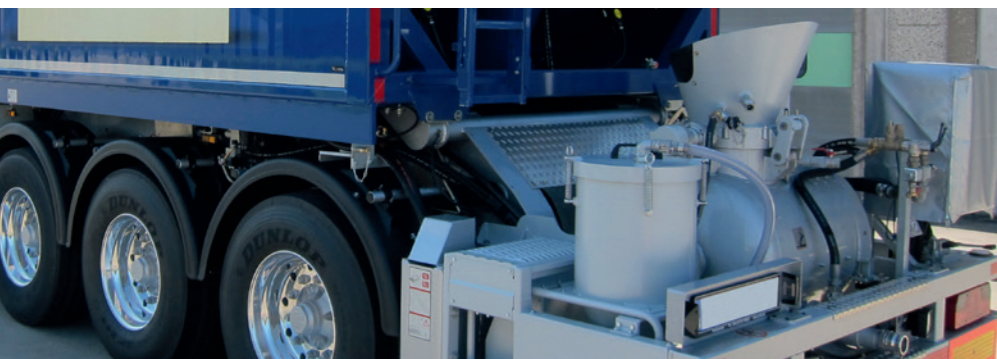
Semi-dry floor screed – mixing chamber with compressed-air conveyor (TransMix 5500)
