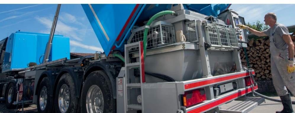
Self levelling floor screed – mixer, feed hopper and worm pump (TransMix 3200)
